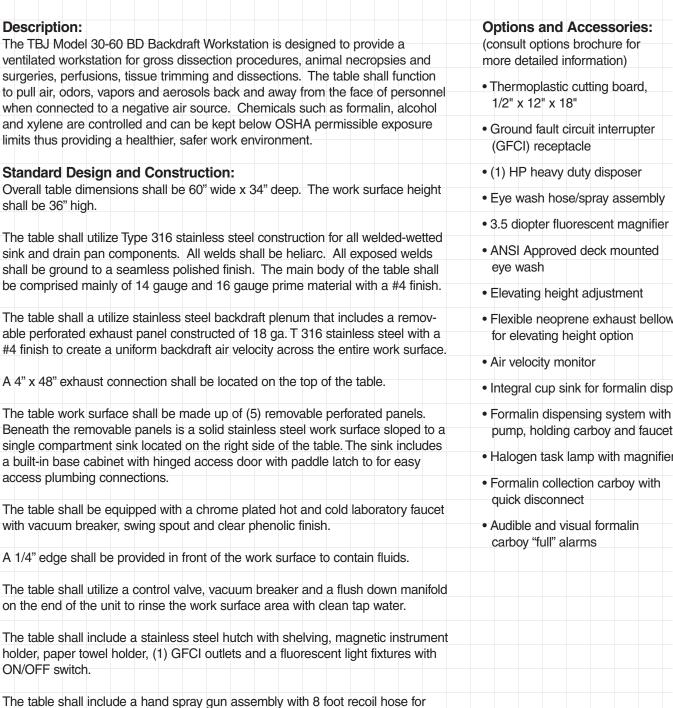
The table shall be factory pre-plumbed and pre-wired ready for single point connection of utilities on site.
